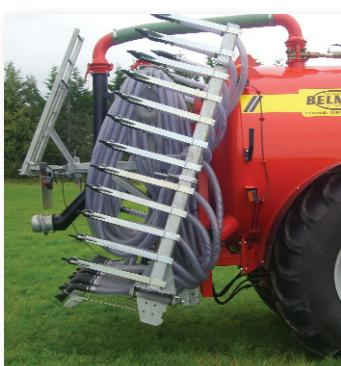
Hoses turn up to prevent remaining slurry leaking out during transport. Fitted with hardened stainless steel trailing shoes and special rubber boots to prevent and minimise blockages. Minimum surface damage occurs with the Belmac trailing shoes.
